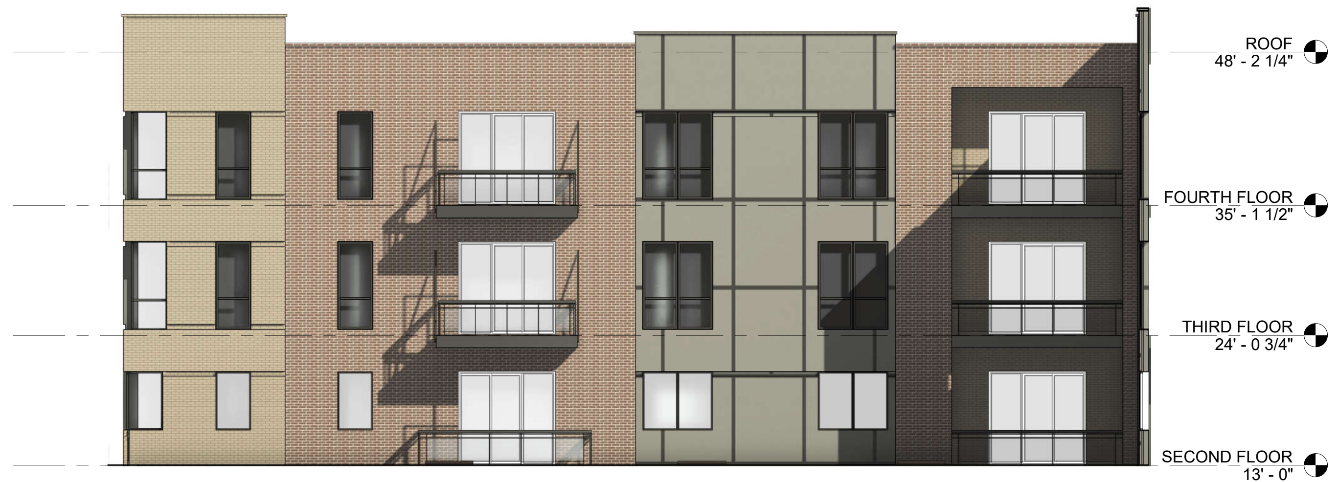
① 2ND FLR TERRACE NORTH FACADE 1/8" = 1'-0" BRICK: 73%; METAL PANEL: 27%
