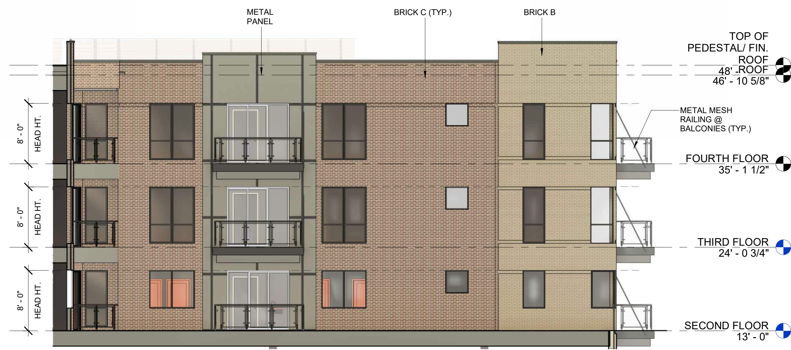
3 2ND FLR TERRACE SOUTH FACADE A102 1/8" = 1'-0" BRICK: 82%; METAL PANEL: 18% (NO LIMIT UNPROTECTED OPENINGS)
