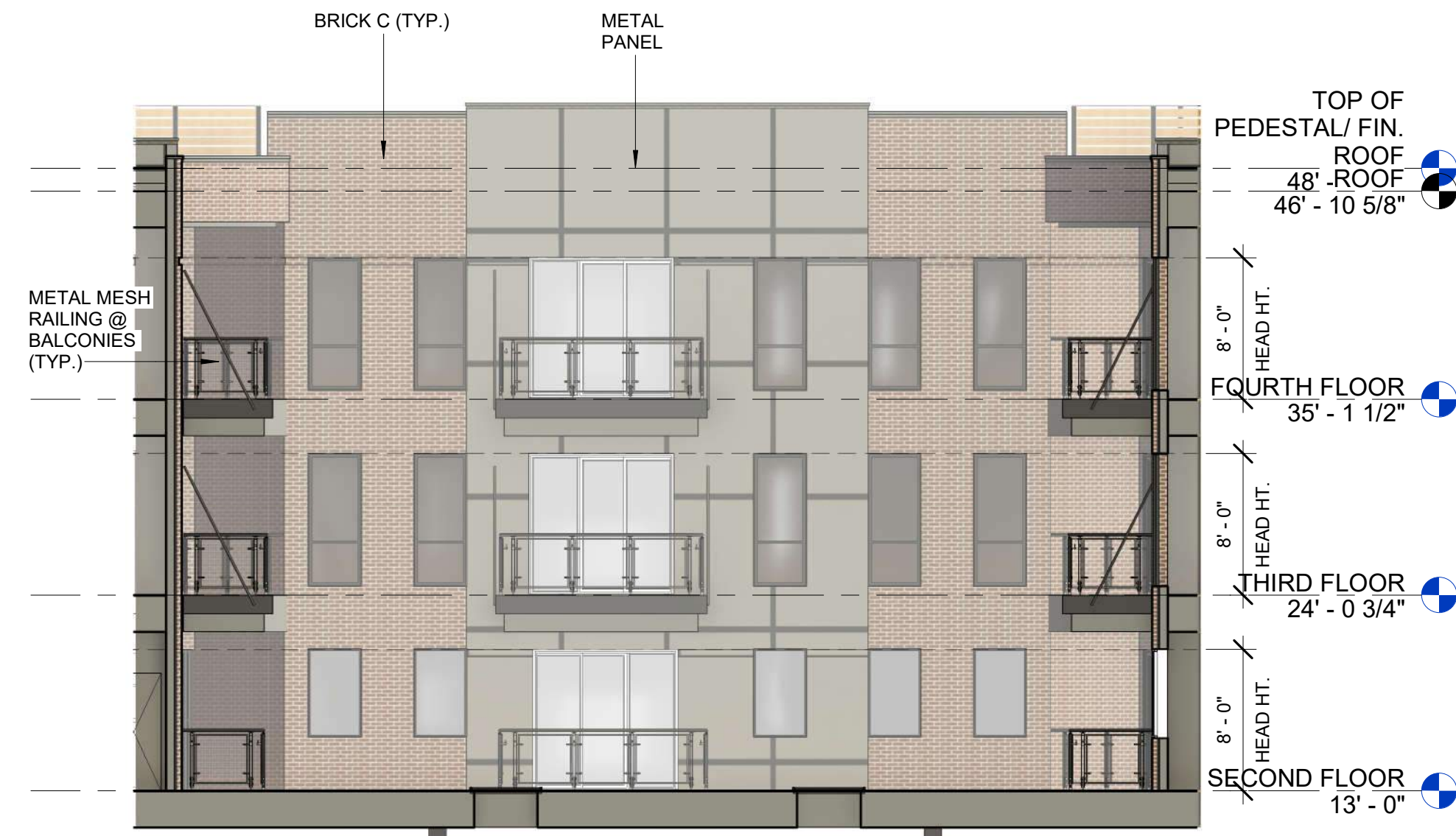
2 2ND FLR TERRACE EAST FACADE A102 1/8" = 1'-0" BRICK: 60%; METAL PANEL: 40% (NO LIMIT UNPROTECTED OPENINGS)
