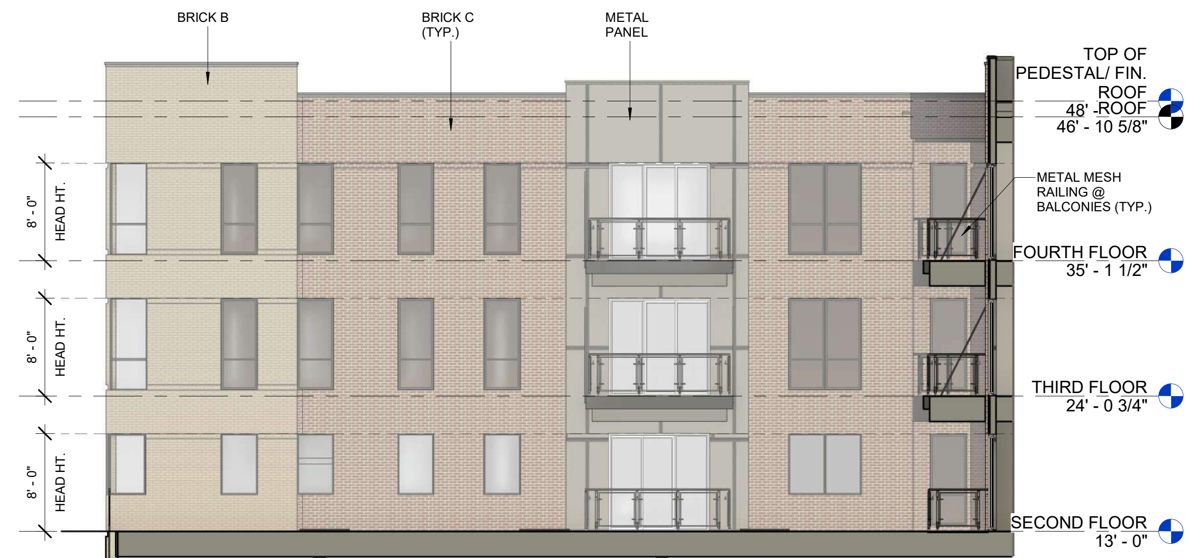
1 2ND FLR TERRACE NORTH FACADE A102 1/8" = 1'-0" BRICK: 82%; METAL PANEL: 18% (NO LIMIT UNPROTECTED OPENINGS)
